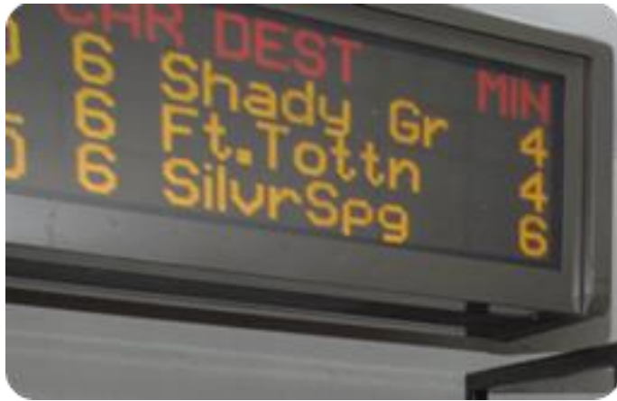
Photo 9: PID display in the DC Metro shows the expected arrival time of the next three trains.
